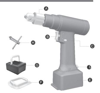
6. Push switch to Forward or Reverse position (C), depress Variable-Speed Trigger to operate handpiece . (B)
