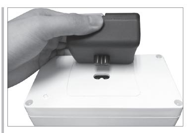
3. The status LED will stay RED until battery pack is fully charged and when the charging is completed, the status indicator will turn GREEN.
