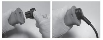
3. Put power cord another end plug into power console" socket. Switch Power ON for ready the operation.
